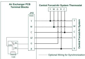
These connections must be done if you want the unit to force the central forced-air system blower operation when ventilating (refer to solid lines in above diagram).
