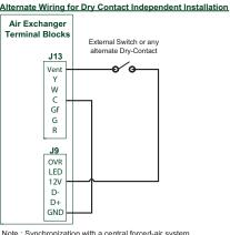
Note: Synchronization with a central forced-air system with W and Y is not available with this configuration
